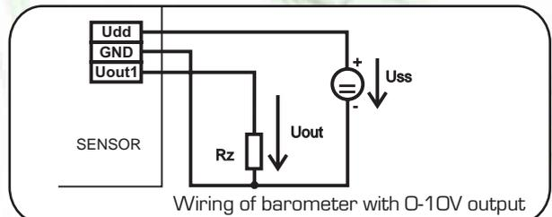
Wiring of barometer with 0-10V output
