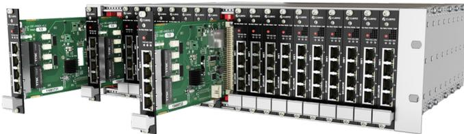
The Cubro FlexTAP B 10/100/1000 allows the uninterrupted passage of full duplex data over standard Category 5/6 copper network cable. The FlexTAP features auto negotiating between 10Mbps, 100 Mbps and 1000 Mbps. The TAP duplicates the network signals, including any existing physical errors, to the transmit-only monitoring ports.
