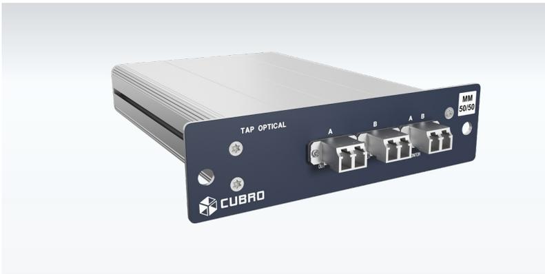
Cubro Optical TAPs offer real-time monitoring access to a physical optical data link with zero performance degradation or disruption. Since an optical TAP is fully passive (no power supply needed) there is no risk associated with placing them inline on an active link. The TAPs do introduce additional optical power loss on the active link which varies with the split ratio used; otherwise, the TAP is completely transparent to the network.
