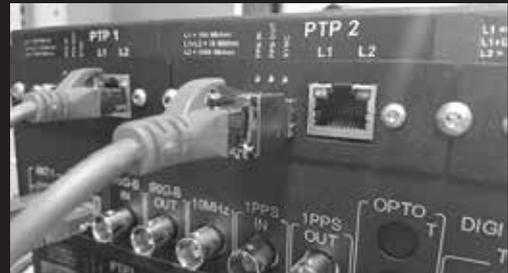
This is back view of Time Server with 1-4 Expander cards. Cards are autonomous GRANDMASTERS. Only card #1 can be set to operate SLAVE mode, but all 4 can act MASTER. Cards support PTP profiles: DEFAULT, ENERGY, TELECOM. The National Physical Laboratory in London (UK) confirms 50ns accuracy of synchronization to cesium clock UTC-NPL.
