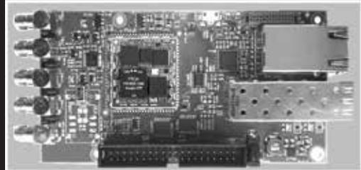
On the right side are output pairs of LAN3-4, 5-6, 7-8, 9-10. On the left side there are internal analogue sync interfaces. They are internally connect via analogue signals SyncBUS.
