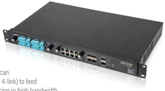
XX-32G features 4 SFP 1G and 2 SFP+ 10G ports. It can accommodate an optional Connectivity Module, providing 8 additional 1 Gbps ports (copper/fiber, SPAN/In-Line). It can also be augmented with an Expansion Module hosting an in-line LC fiber optic TAP (1- or 4-link) to feed into the SFP SPAN Module ports, providing aggregation, routing, filtering and load balancing in high bandwidth port monitoring and analysis scenarios.
