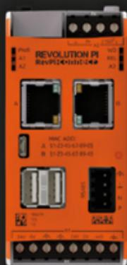
Compact DIN rail housing with a width of just 45 mm
