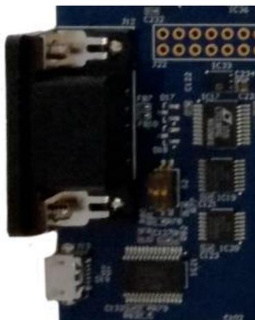
Figure: Dsub9 and micro USB port for serial interface
