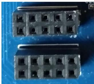
Figure: SPI header and Fast SPI header
