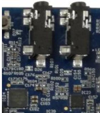
Figure: HDA (left) and I2S (right) 3.5 mm sockets
