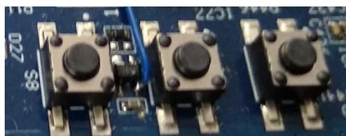
Figure: System reset (left), CPU reset (middle), and reserved (right) buttons
