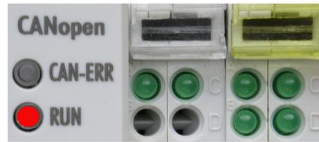
For a consistent state or error indication respective error diagnosis of CANopen devices the module *LED* is available. It is included in the default delivery of the *CANopen Library*.
