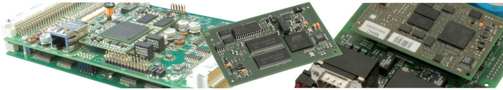
The PLCcore SOM is an insert-ready, OEM-able single board computer subassembly, coming with a state-of-the-art operating system and IEC 61131-3 runtime kernel pre-installed on the module. Performance-optimized 32-bit CPU core components, value-adding peripherals and the fully customizable I/O layer makes the PLCcore a truly generic platform for own control application developments.
